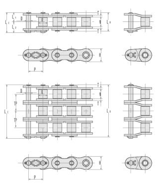
SY Heavy series roller chains are designed with thicker side plates to insure greater capacity for absorbing shock loads without fatigue failure of side plates. Also manufactured to close tolerances in accordance with ANSI specifications and are mainly used for applications where space and design limitations prohibit the use of a large size roller chain, and yet greater load carrying capacities are needed in oil-field drilling operations.
